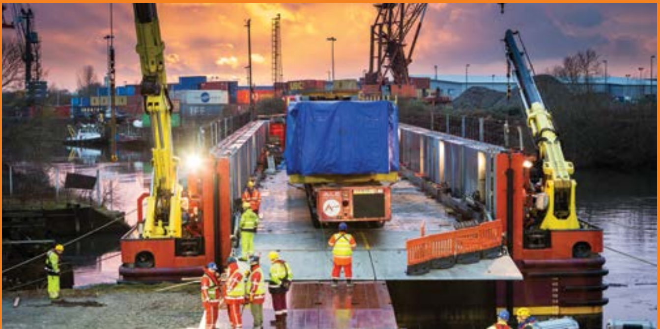
Manchester Ship Canal was used for the delivery of oversized loads, avoiding road congestion issues and the cause of disruption to local traffic movements.
