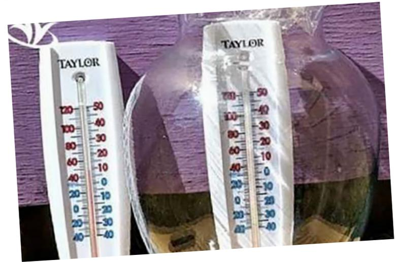
Global warming is a key component of climate change, and it is caused in part by an enhanced greenhouse effect. Climate change activities like this one show us just what that term means. Place two thermometers side-by-side in a sunny spot. Put one inside a covered glass jar and leave the other one outside. Observe the temperatures after about 20 minutes to see which is higher.
