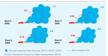
FIGURE 18: LABORATORY AND ACTUAL ROAD EMISSIONS OF NITROGEN OXIDE COMPARED (NO, IN g/km)
