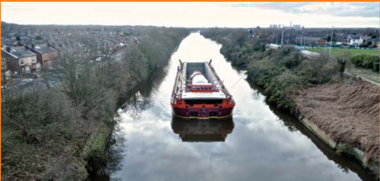
The Terra Merique delivered over 8000 tonnes of plant and equipment to site via the Manchester Shipping Canal (Gas Turbines, Generators, HRSGs, Condensers).
