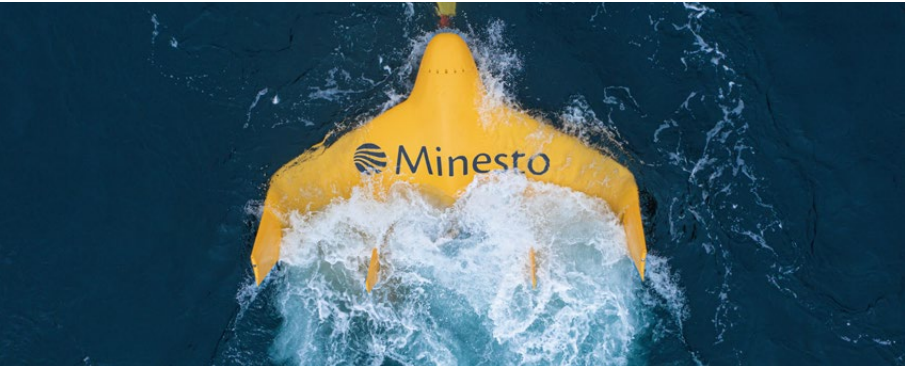
Tidal energy device harnessing power from ocean currents (Credit: Minesto)
