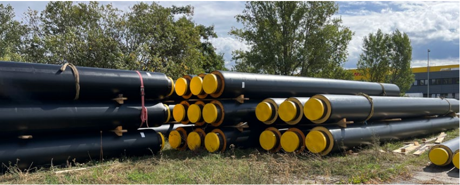
District heating pipes ready to be laid in Germany
