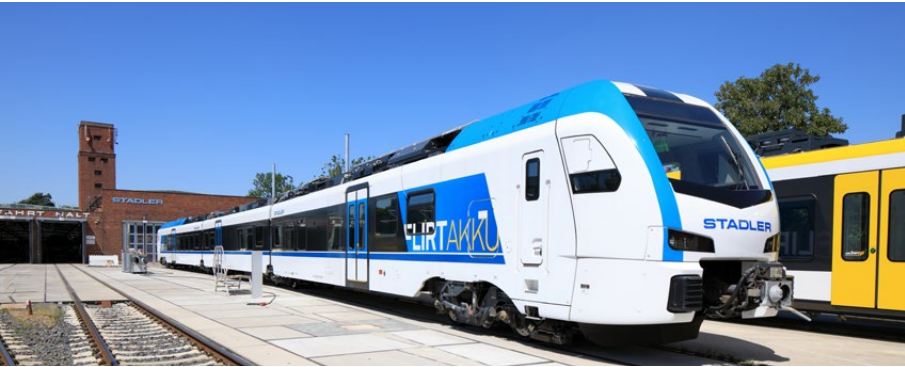
Stadler battery electric train designed to operate on regional routes with non-electrified sections (Credit: Stadler)
