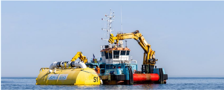
Seaturns wave energy converters undergoing sea trials off France's Atlantic coast (Credit: Christophe Beyssier & Seaturns)
