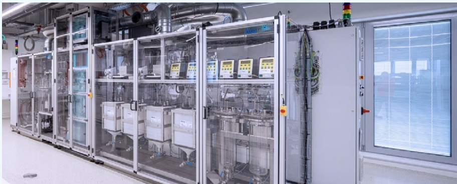
Lab-scale precipitation reactor for the development of an active material for sodium-ion batteries (© Fraunhofer IFAM)
