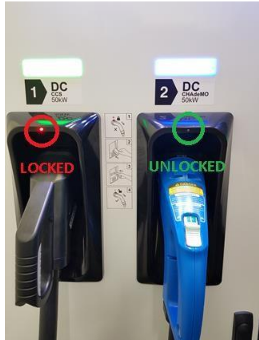
Figure 7. CHAdeMO Connector unlocked
