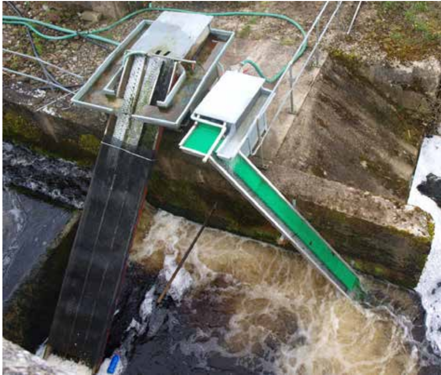
The 'new' and 'old' juvenile eel traps located on the Co. Tipperary bankside of Parteen Regulating Weir.
