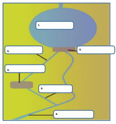
Look out along the canal leading to the dam. This is called the headrace canal. 12km away is Parteen Weir and behind it is Lough Derg. Once the water passes through Ardnacrusha it follows the tailrace canal (the lower outgoing canal) to rejoin the River Shannon.
