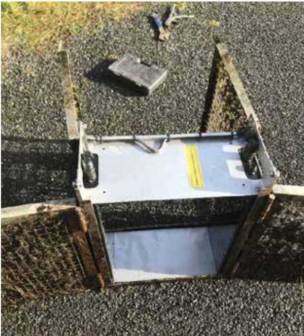
The stainless-steel inscales and new fish counter frame and scanning unit ready for installation.
