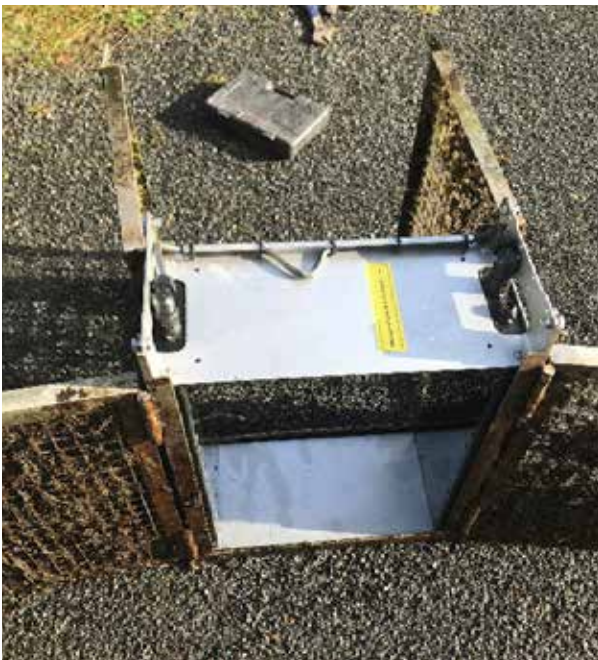
A stainless steel inscales with a new scanning unit inserted. In late December 2021, this unit was overhauled and will be used to assess fish movements and census data at Gweedore Regulating Weir which is located on the Clady River.
