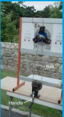
This is the simplest form of creating electrical energy - spinning a magnet inside a coil of copper wire. In this case the spinning creates just enough electricity to light a single light bulb.
