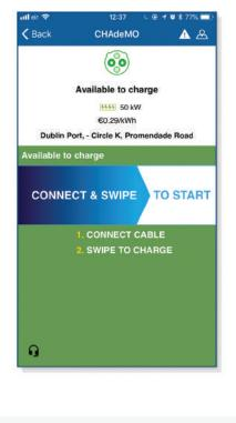
To start a charge, connect the cable and swipe right Remember to check the app
