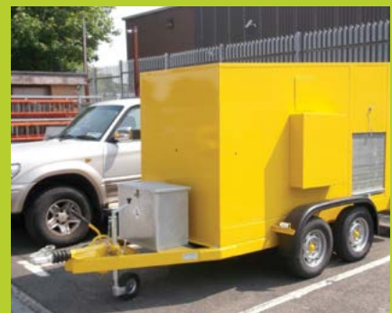
Top: Typical Oil Storage Facility after improvements Above: Mobile Bunded Bowser
