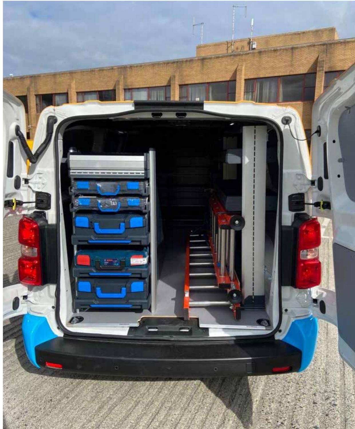
ESB Networks Fleet & Equipment have also worked closely with operational end users within the business to design a bespoke lightweight internal fitout for tool and spare part storage as well as an internally stored ladder, to promote vehicle efficiency and improve vehicle range.
